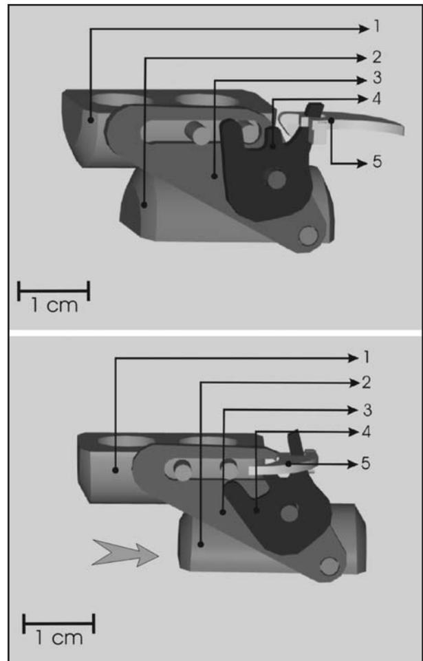
Fig. 3: 1- Upper anchor splint; 2- Lower anchor splint; 3- Inner sliding plate; 4-Outer sliding plate;; 5- Commissure wing. Top: in resting position. Bottom: during movement.
