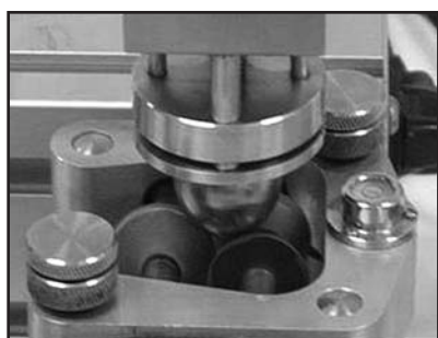
Fig. 1: The metal sphere on the wear machine rollers.
