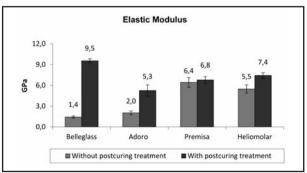
Fig. 2: Modulus of elasticity of direct and indirect composites without and with post-curing treatment.
