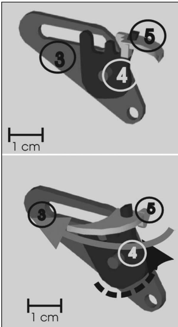
Fig. 2: Inner (3) and Outer (4) sliding plates and Commissure wing (5). Primary mechanism (dotted arrow); secondary mechanism (full line arrow). Top: in resting position. Bottom: during movement.
