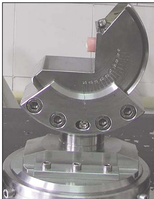
Fig. 3: Device for mounting on the universal testing machine.
