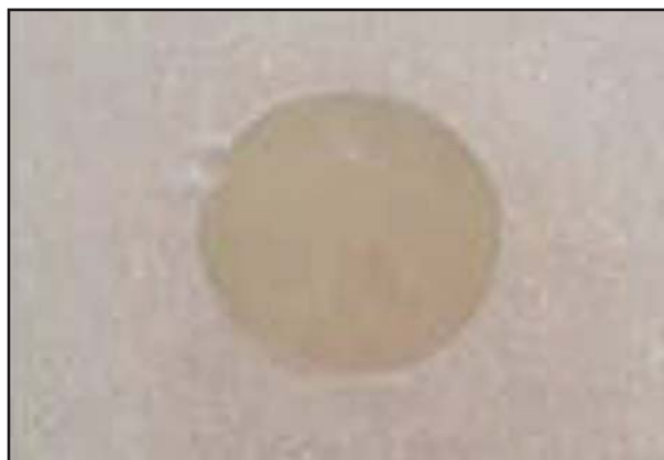
Fig. 5: Adhesive paper with a perforation of the same diameter as the ceramic test cylinders covering tooth surface to limit the adhesion area.
