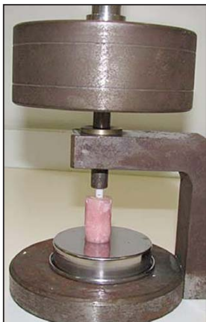
Fig. 6: Ad-hoc standardizing device for cementing force, applying a constant 25N load.
