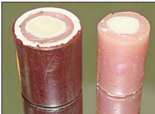
Fig. 2: Specimens embedded in acrylic resin to be mounted on the universal testing machine.
