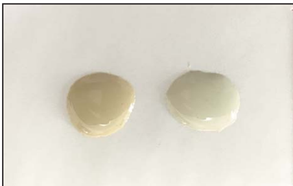
Fig. 1: The base and catalyst pastes of a calcium hydroxide cement were dispensed at a 1:1 ratio (conventional technique).
