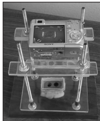
Fig. 5: Top view of impression positioner in the ad-hoc device.
