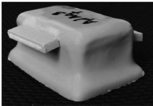
Fig. 2: Custom tray made of thermoplastic sheet.
