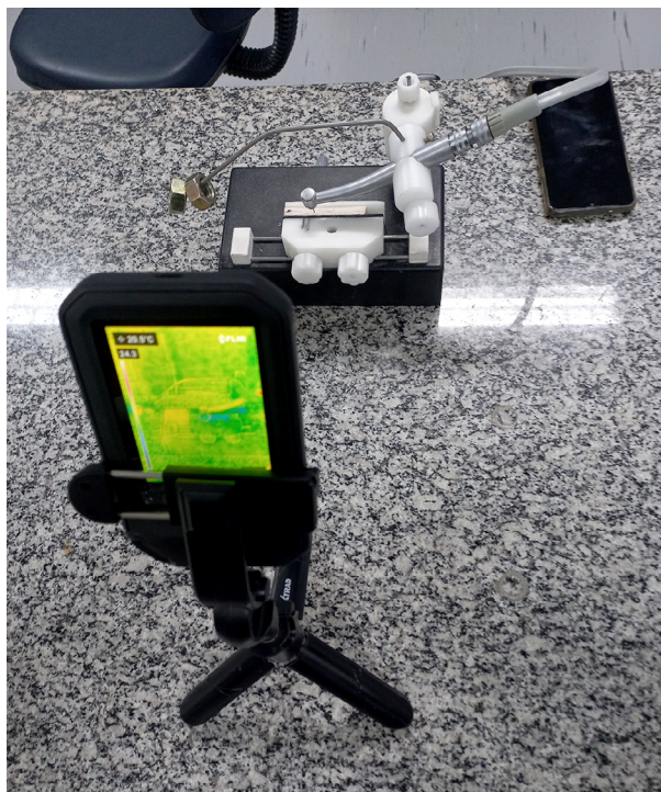
Fig. 5: Position of the infrared thermographic camera during the experiment.
