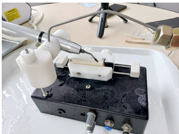
Fig. 4: Position of the insert with “spray control” in the automated cutting device.
