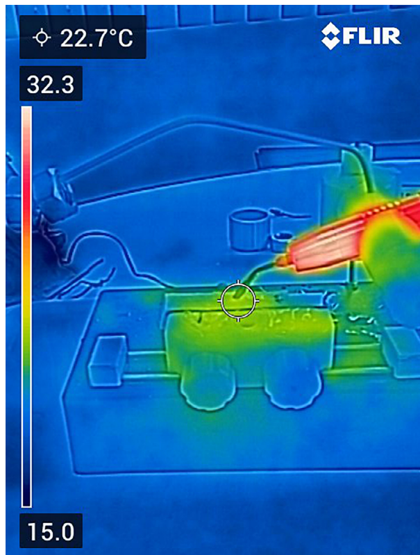
Fig. 6: Thermal image obtained during the osteotomy performed with the ultrasonic insert. Piezoelectric insert positioned over the bone block, which was attached to the automated cutting device. The photo was taken by the thermographic camera at the time the osteotomy was performed and shows the temperature of the delimited target.
